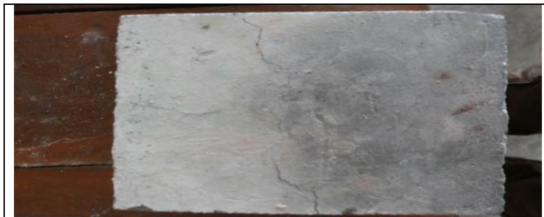
Figure 6 : Copper slag Concrete after exposed to 600 o C.
