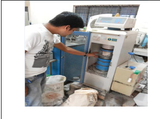
Figure 4: Compressive Strength Test Setup in CTM
