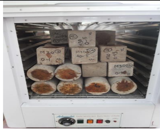
Figure 5: Concrete Specimens Subjected to Elevated Temperature
